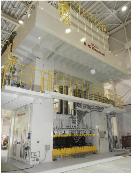
Fig. 3. Large high-speed hydraulic press of 3500 ton weight capacity installed in national composites center Japan in 2013: Key facility for LFT-d technology.
